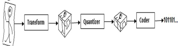
Fig1. The three steps of digital image compression system
