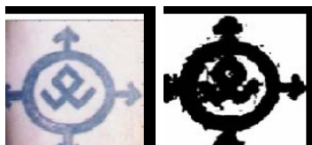
Fig. 7: Skin detection: a) original image; b) skin shown in white and potential tattoo area in black.
