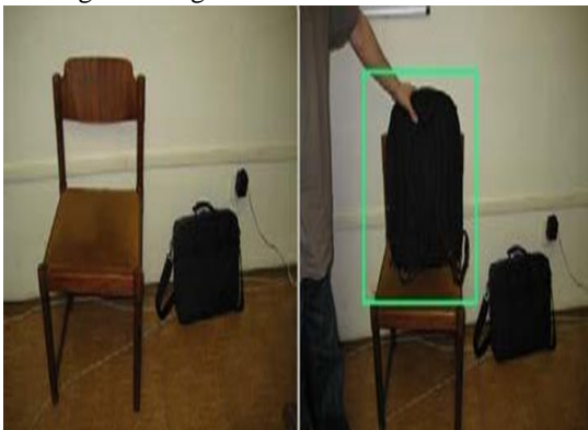
Fig. 3 a) Detection of one luggage b) Detection of one abandoned luggage
