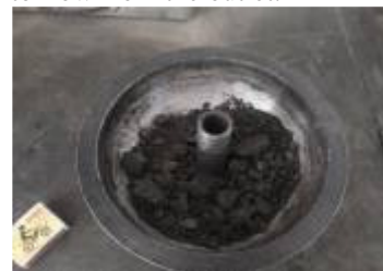
Fig.8 RAP Aggregates after bitumen extraction
