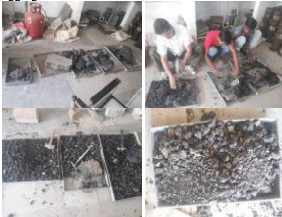
Fig.5 Breaking of RAP aggregates with the help of hammer
