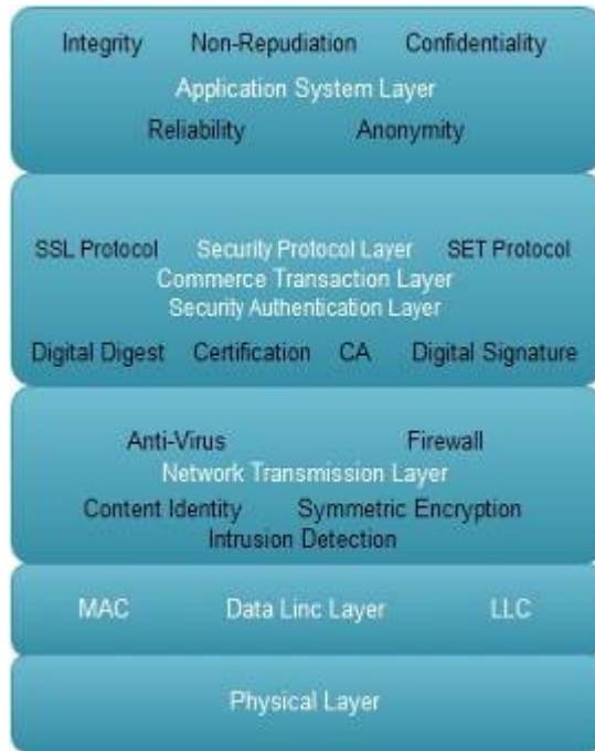
Fig 1: Architecture of EC Security Technology
