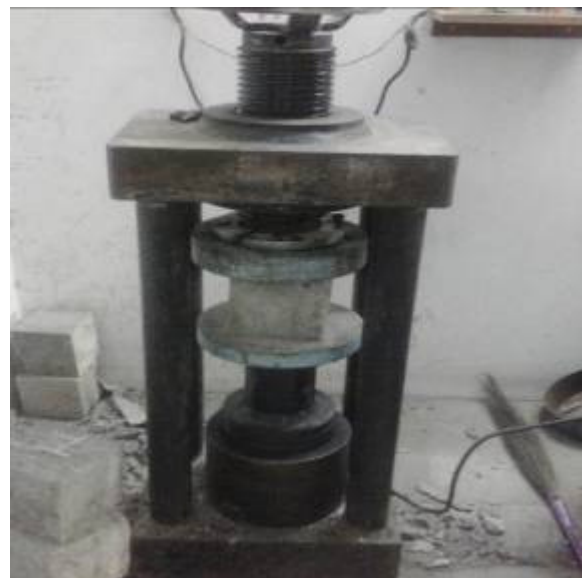
Fig. 2: Test for Compressive Strength
