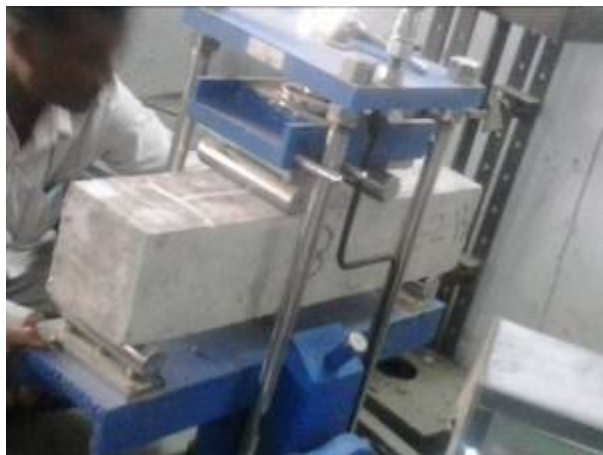
Figure 3: Test for Flexural Strength of Concrete
