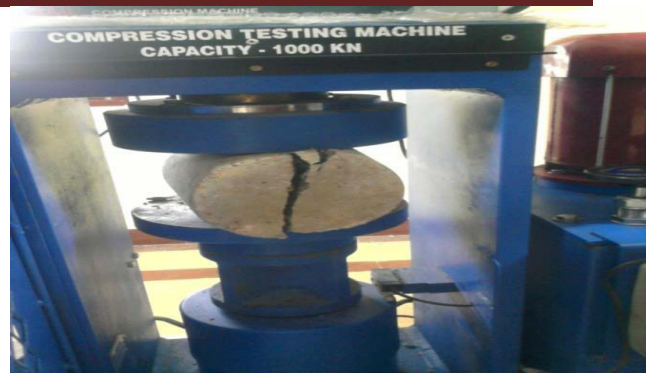
Figure 4: Test for Splitting Tensile Strength
