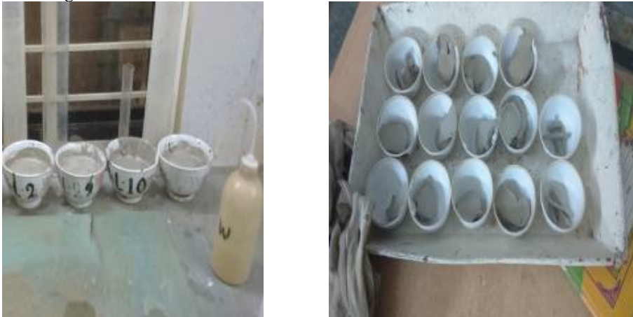
Figure 5.1 Test Specimen of Plastic and Liquid limit
