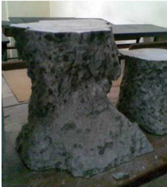
Fig. 7.3 Ultimate Cracking pattern of Cubes
