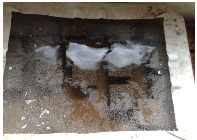
Figure 2 Curing of concrete blocks for 14 days
