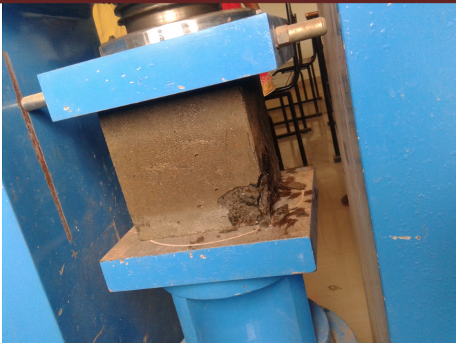
Figure 3 Compression load of 580 KN applied on the block
