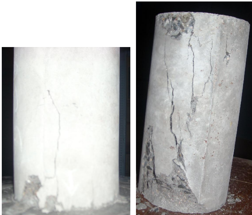
Fig.11 Nucleation of inclined fracture surface and diagonal fracture zone
