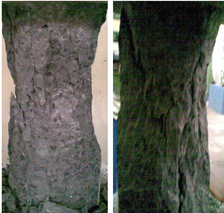
Fig.12 Ultimate Cracking pattern in cylinders
