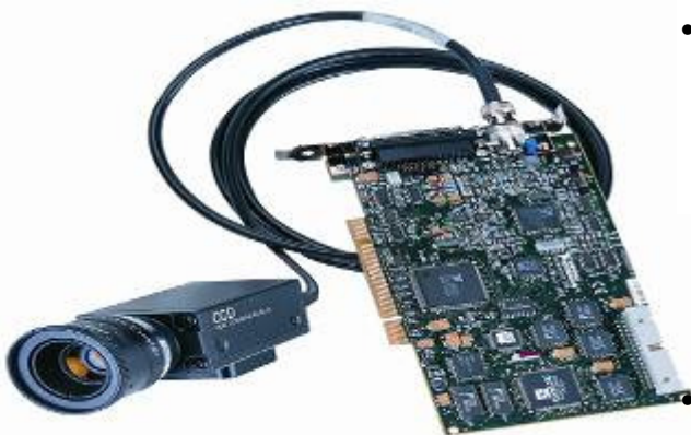
Figure.1 Typical high cost frame grabber connected with video camera
