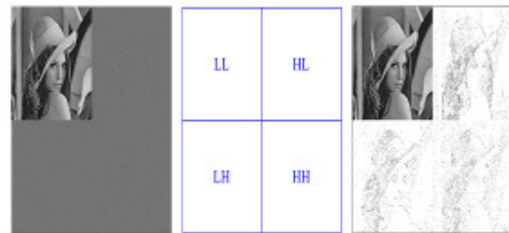
Fig. 1 one dimensional CDF (2,2) wavelet transform applied to the rows of the benchmark image lena with reflection at the image boundaries[3]
