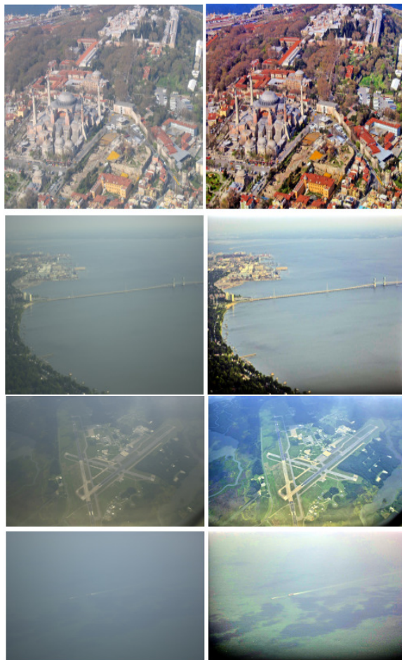
Figure 2 The enhancement results for different types of turbidity. Left Column is of original images. Right column Enhanced images.
