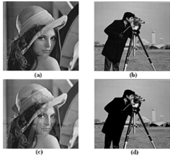
Fig. 3. Shows (a) Lena image (b) Cameraman image to be Watermarked (c) visible watermarked Image and (d) the recovered cameraman image.
