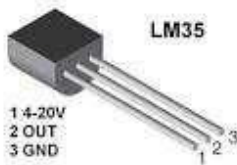
Fig.3 Temperature sensor LM 35
