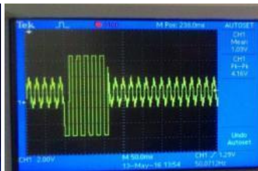
Fig.14. Current waveform for A- phase under L-G fault condition
