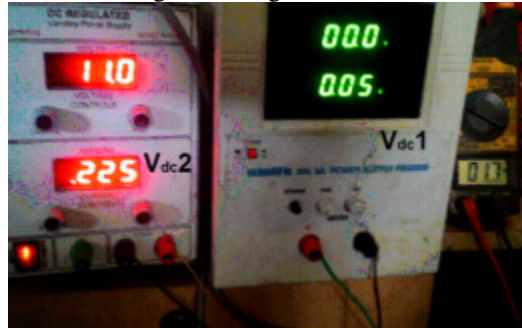
Fig.20 State 3 input and output voltage
