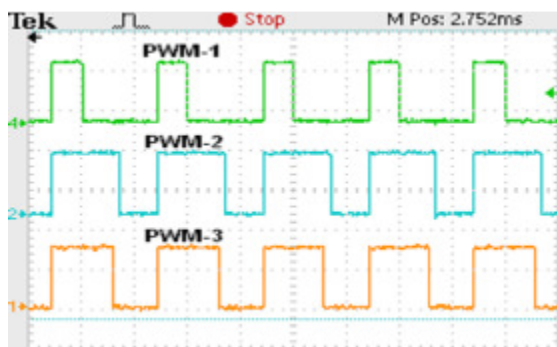
Fig.6(a) Generated gate pulses for three upper switches. (Scale: x-axis:25usec/div, y-axis:2V/div)
