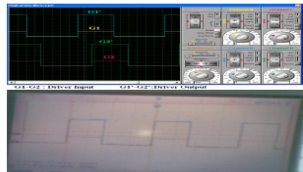
Figure 13. Comparative Result for Driver circuit input and output waveform
