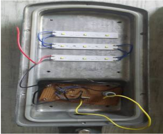
Figure 3.4 LED driving circuit
