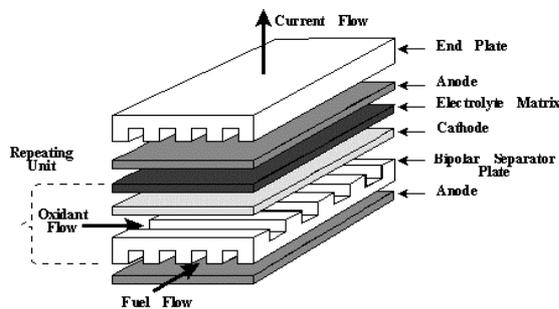
Fig. 2 Working Of Fuel Cell
