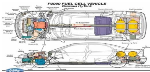
Fig. 4 Fuel Cell Vehicle
