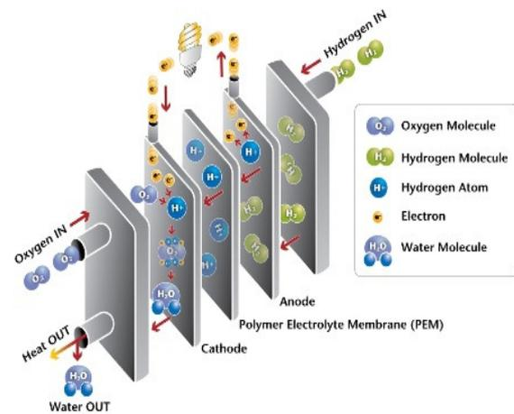
Fig. 3 Fuel Cell Stack
