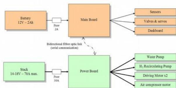
Fig. 6 Diagram of Electric Supply
