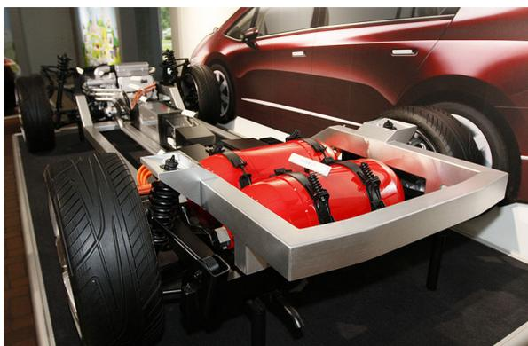
Fig. 5 Gaseous H<sub>2</sub> Tank
