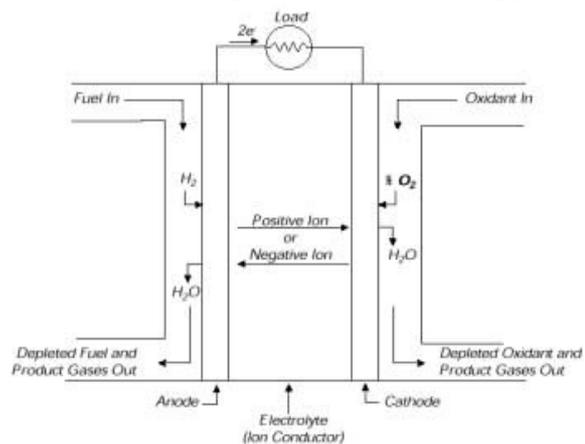
Fig. 1 Schematic of an Individual Fuel Cell
