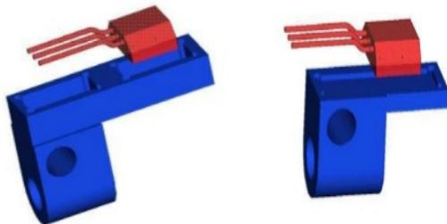
(a) Slider for the MP joint. (b) Slider for the DIP joint.
