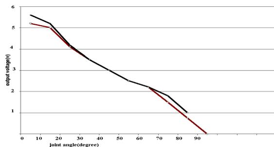
Fig. 10:- Calibration curve of the joint angle
