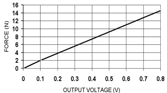
Fig. 11:- Calibration curve of the force sensor
