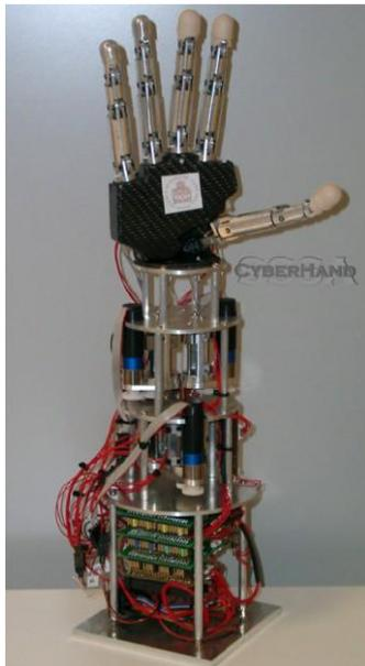
Fig.6-: The socket containing motors and control electronics.
