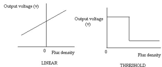
**Fig. 8:- Calibration curve of the effect sensor**
