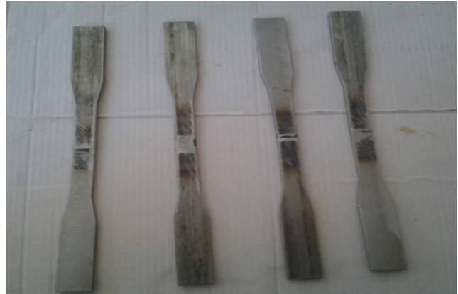
Figure 6. Specimen before fatigue failure
