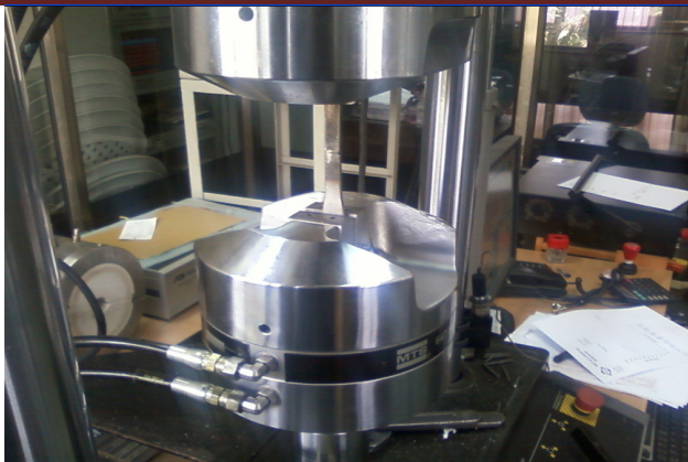
Figure 4. Fatigue Testing of Specimen loaded on MTS machine
