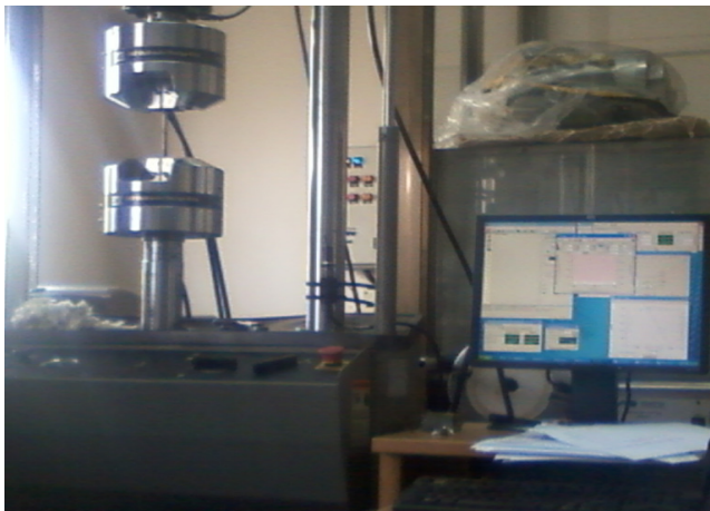
Figure 5. Fatigue Testing of Specimen on MTS machine with Software Interface
