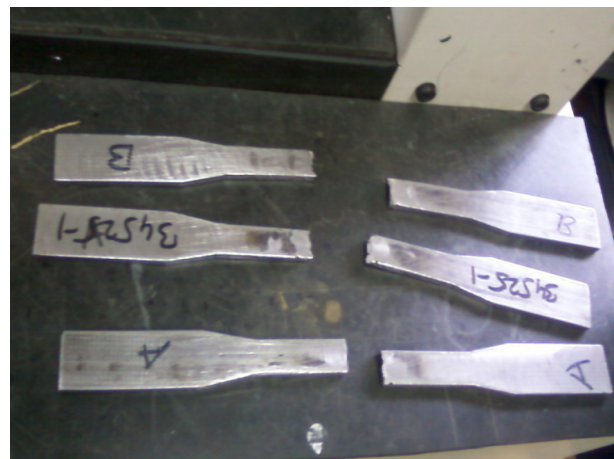
Figure 7. Specimen after fatigue failure.
