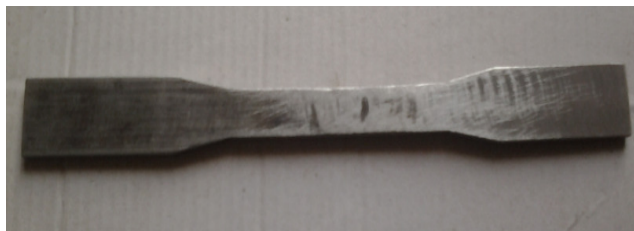
Figure 2. Specimen prepared for fatigue Testing
