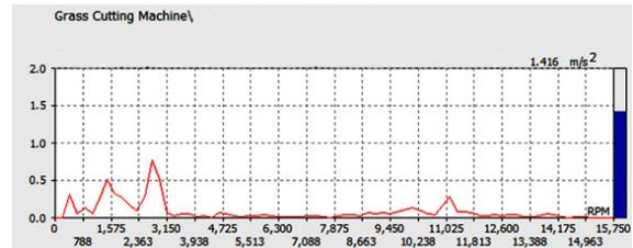
The following table 7.2 shows the acceleration level for different cutter speed, which is well below the daily exposure limit as well the vibration level is reduced as compare to the existing grass cutter.
