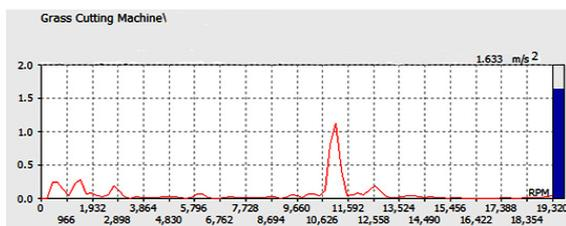
The above fig7.10 shows the amplitude of vibration for the cutter speed 2800 rpm. The amplitude of vibration is 1.633 m/s<sup>2</sup>.
