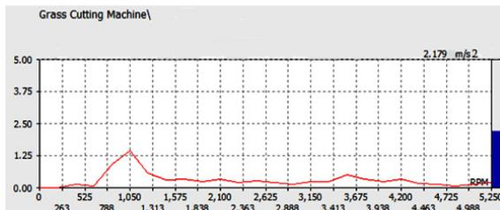
The above fig 7.9 shows the acceleration amplitude for the cutter speed 3200. The amplitude is 2.179 m/s<sup>2</sup>
