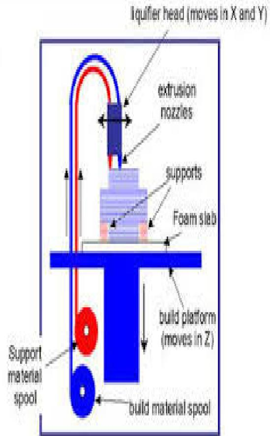
FIG: FUSED DEPOSITION MODELING
