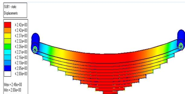
Fig.4 Displacement in steel leaf spring using hyper mesh
