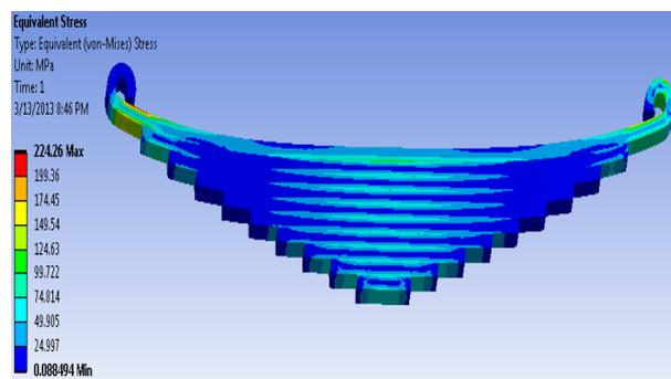
Fig.1 Von misses stress in steel leaf spring using Ansys
