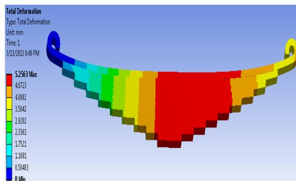
Fig.2 Displacement in steel leaf spring using Ansys
