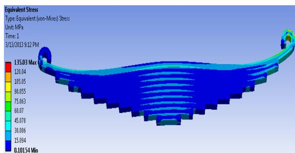
Fig.5 Von misses stress in multi composite leaf spring using ANSYS
