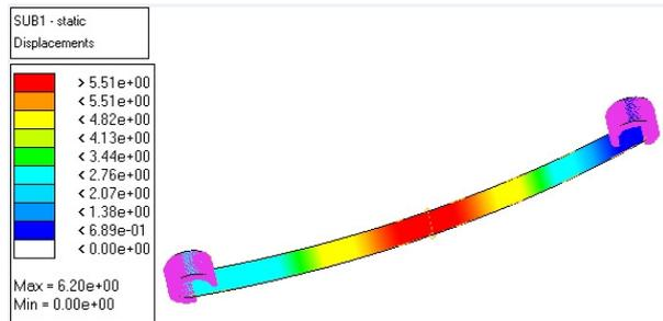
Fig.8 Displacement in mono composite leaf spring using hyper mesh
