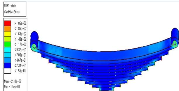
Fig.3 Von mises stress in leaf spring using Hypermesh
