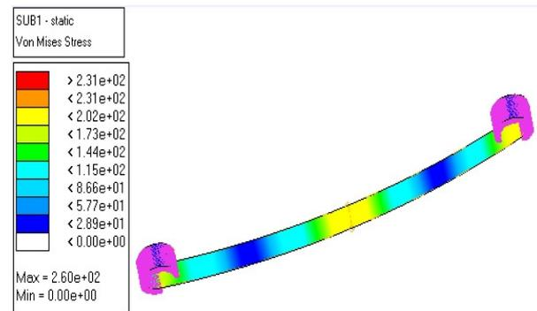
Fig.7 Von-misses stress in mono composite leaf spring using hyper mesh
