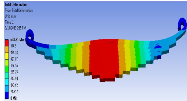
Fig.6 Displacement plot in multi composite leaf spring using ANSYS
