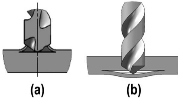
Fig.1: Delamination mechanisms: (a) Peel-up and (b) Push-down<sup>[11]</sup>
