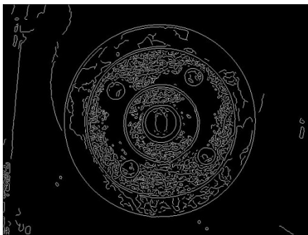
Fig 5. Edge Detection of pulley using Canny Operator.
