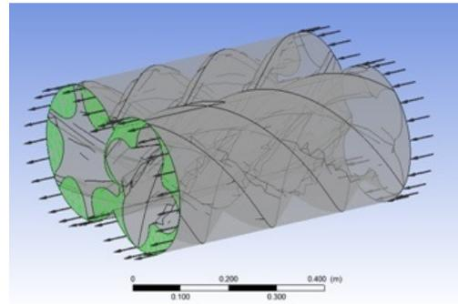
Figure 3. Rotary air compressor cavity model with inlet and outlet
