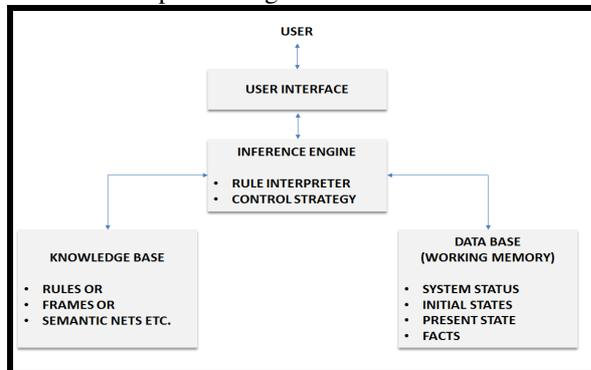
(Figure 4: Expert System schema)
