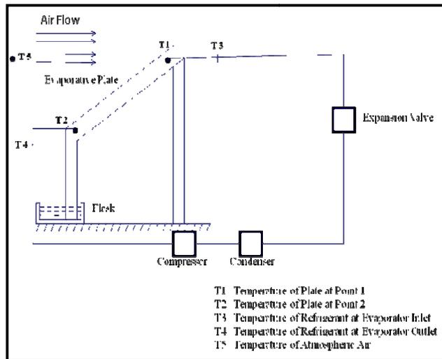
**Figure 2.1 Set up diagram**
