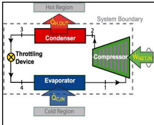
**Figure 2.2: Vapour Compression System**
