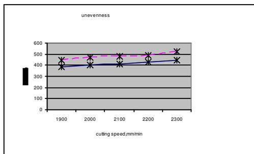
Fig-3: Cutting speed Vs unevenness of 12mm plate thickness
