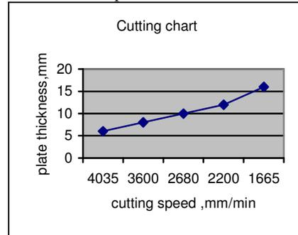
Fig-2: Cutting speed Vs Plate thickness of EN-9 - 400 materials
