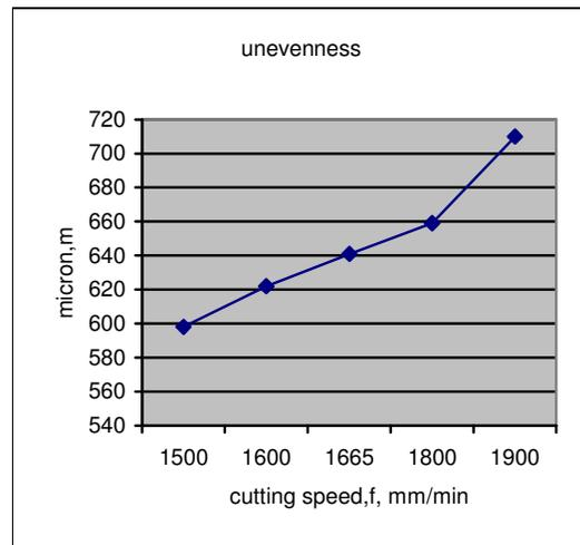
Fig-4: Cutting Speed Vs Unevenness
