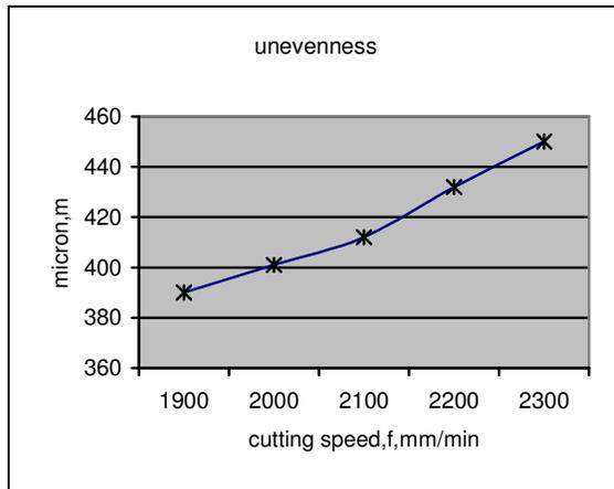
Fig-5 Ref. [3] cutting speed Vs unevenness
