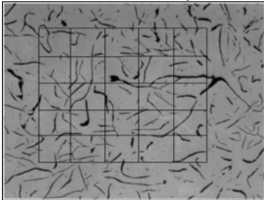
Fig.2 Measurement of area percentage of phases in gray cast iron by point count method
