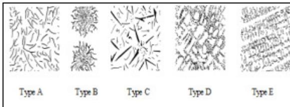
Fig 1. Types of graphite flakes distribution in gray cast iron as per ASTM A247.
