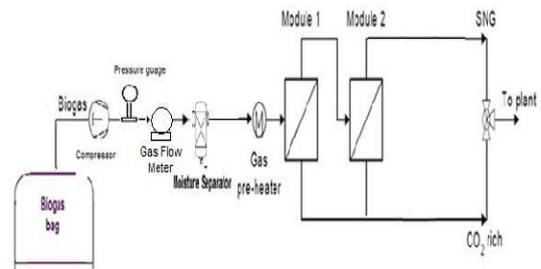
Fig. 4 Block Diagram of Separation of CO<sub>2</sub> gas from Methane Gas
