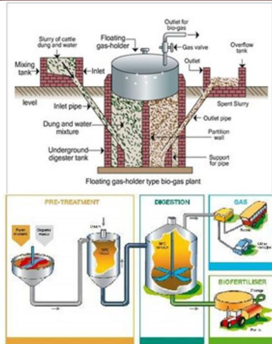
**Fig. 2 Production Process for Methane Gas**
