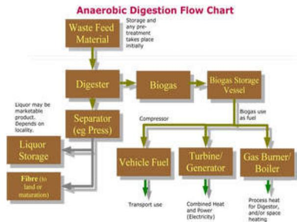
Fig. 1 Anaerobic Digestion Flow Chart
