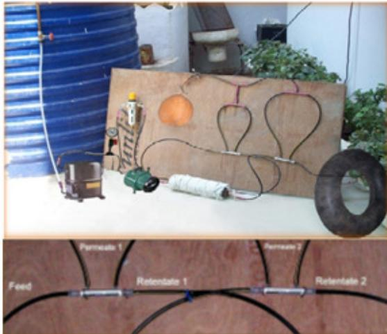
Fig. 3 Setup of Separation of CO<sub>2</sub> from Methane
