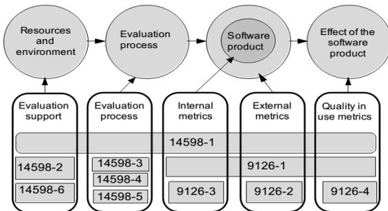
Figure 2: Current architecture of ISO/IEC 9126 and 14598 series
