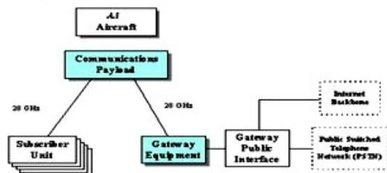
Block Diagram Representation of Airborne Internet Network Architecture.
