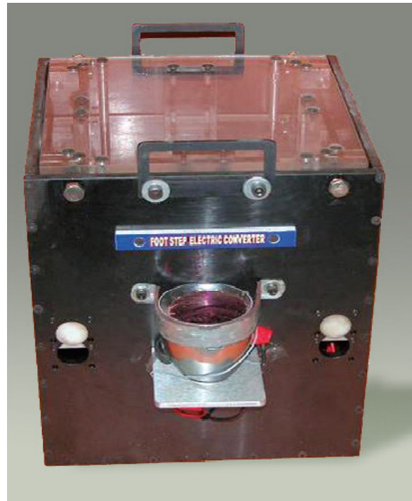
Fig.2. Foot step electric convertor device
