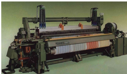
Fig 4.3.1 Lakshmi RUTI-C 1000 shuttle weaving machine
