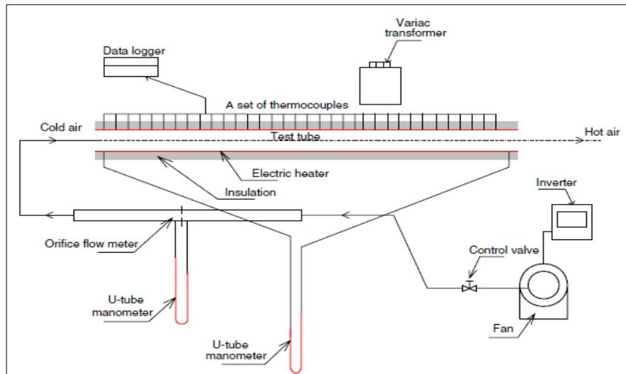
Figure 1 Schematic representation of experimental setup
