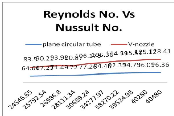
The graph shows the relations between Reynolds no and heat transfer coefficient. The heat transfer coefficient increases with the increase in the Reynolds no. and the friction factor increases in the v-nozzle.
