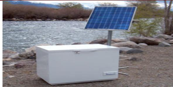
**Figure.3. Set-up of Solar Assisted Refrigeration System**
