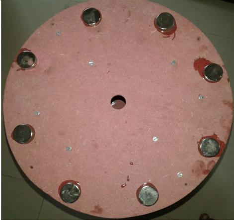
Fig-5 Placement of disc magnets on rotor
