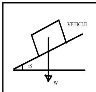
Figure. FBD of Vehicle on Slop
