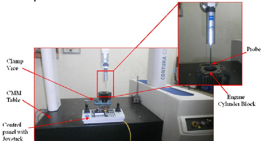
Fig.4.2: Experimental Set-up of CMM
