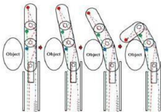
**Fig. Grasping motion of the prosthetic finger**
