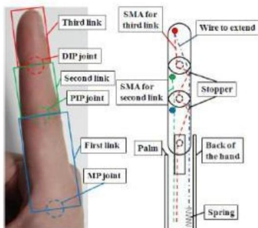
Fig. Structure of human finger and prosthetic finger.
