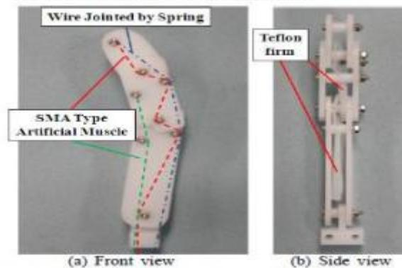
**Fig. First and second prosthetic fingers.**
