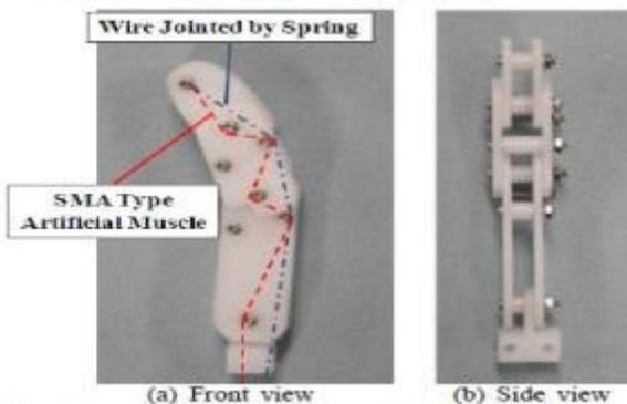
**Fig. The third and fourth prosthetic fingers.**
