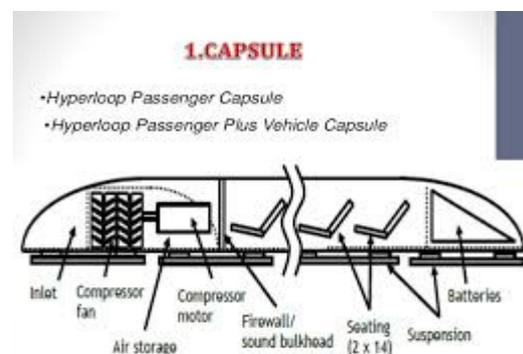
Fig 2. Hyperloop Passenger Plus Vehicle Capsule.
